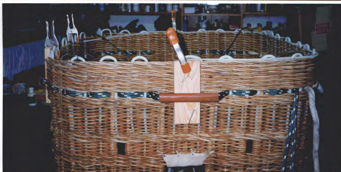
You are looking at the bottom of Wayne Wooster's Colt basket. The basket floor has been removed. Wayne has replaced one, of each pair, of the vertical rattan stakes with nylon rod. Heavier nylon rods are lashed to the verticals with stainless steel wire. The wire wrap appears like silver tape in the photo. Wayne plans to lace the rattan basket to a new floor with steel cable.
